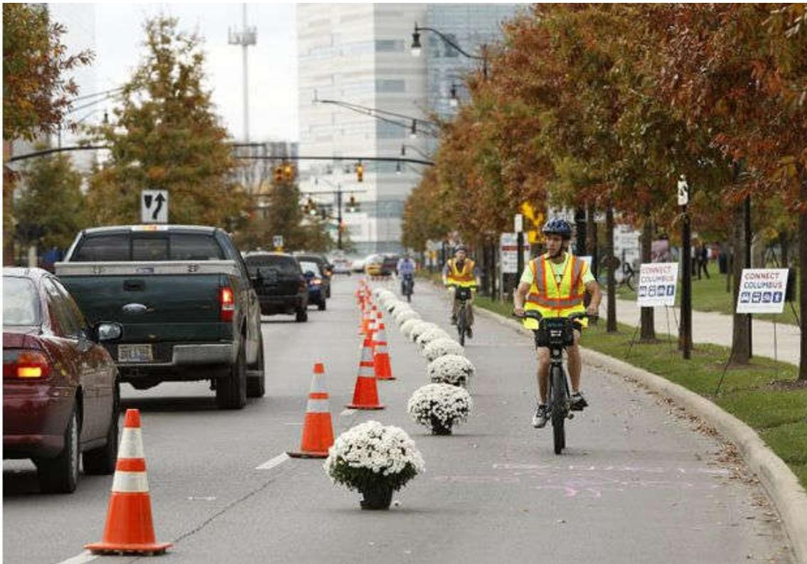
**Image 7:** example of temporary separated bikeline (Source: The Columbus Dispatch).
